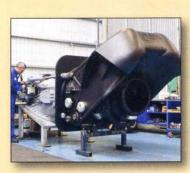
new reverse duct design, reducing the transom footprint. The HT810 is supplied with a factory-built transition duct, eliminating the need for this to be fabricated by the boat builder and ensuring accurate geometry for the intake flow.
