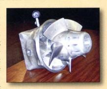
functions like a controllable pitch propeller while retaining the shallow draft, safety and maneuverability of a marine jet. Reverse flow through the jet eliminates the need for a reversing bucket which allows a larger diameter system with higher propulsion efficiency to fit in the same space.
